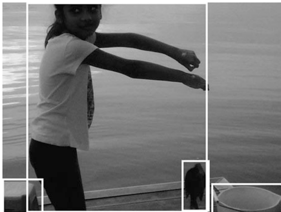
Figure 8.20: Example of object detection. Here, four objects are identified together with their bounding boxes. The four objects are “fish,” “girl,” “bucket,” and “seat.” The image is illustrative only.
