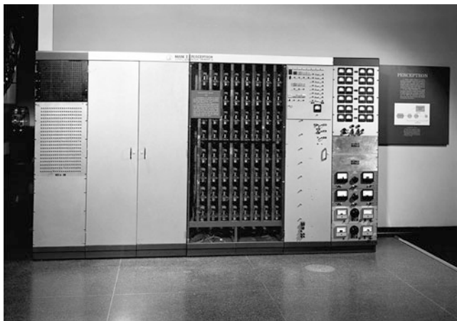
Figure 1.5: The perceptron algorithm was originally implemented using hardware circuits. The image depicts the Mark I perceptron machine built in 1958. (Courtesy: Smithsonian Institute)
