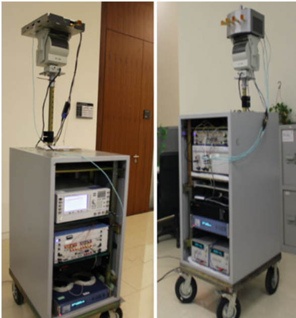
Fig. 1 Channel sounder at E-band, transmitter ( left ) and receiver ( right )
