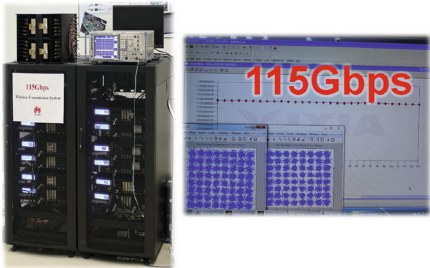
Fig. 8 115 Gbps prototype E-band, transmitter and receiver ( left ), real-time receiver performance ( right )
